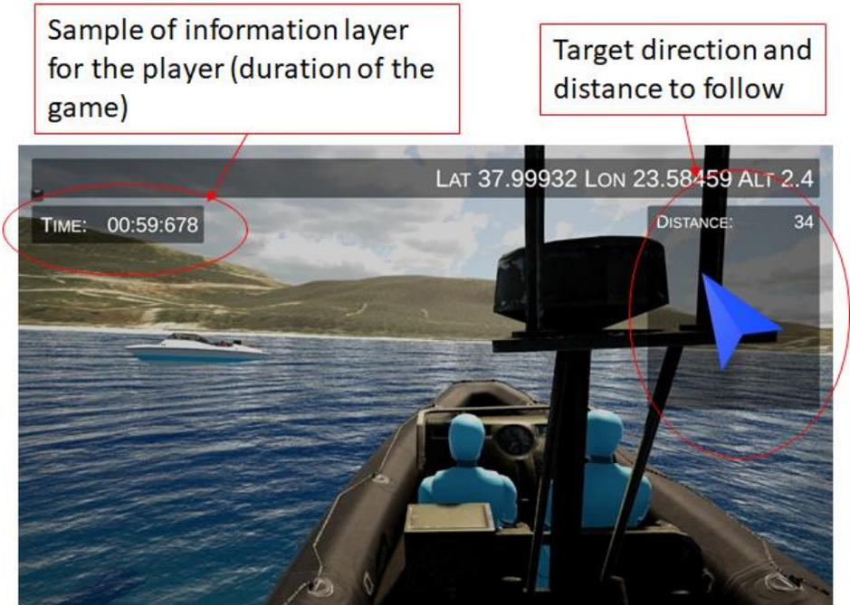
Figure 4: ARESIBO AR interfaces used in the training system.
