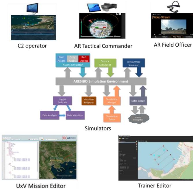
**Figure 3: ARESIBO AR interfaces used in the training system.**
