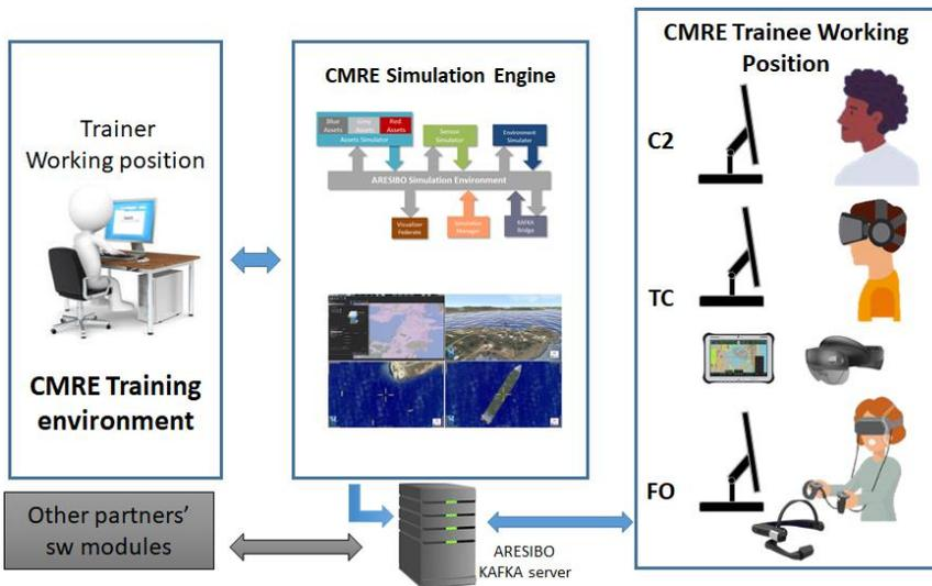
**Figure 2: Simulation based Training System architecture.**
