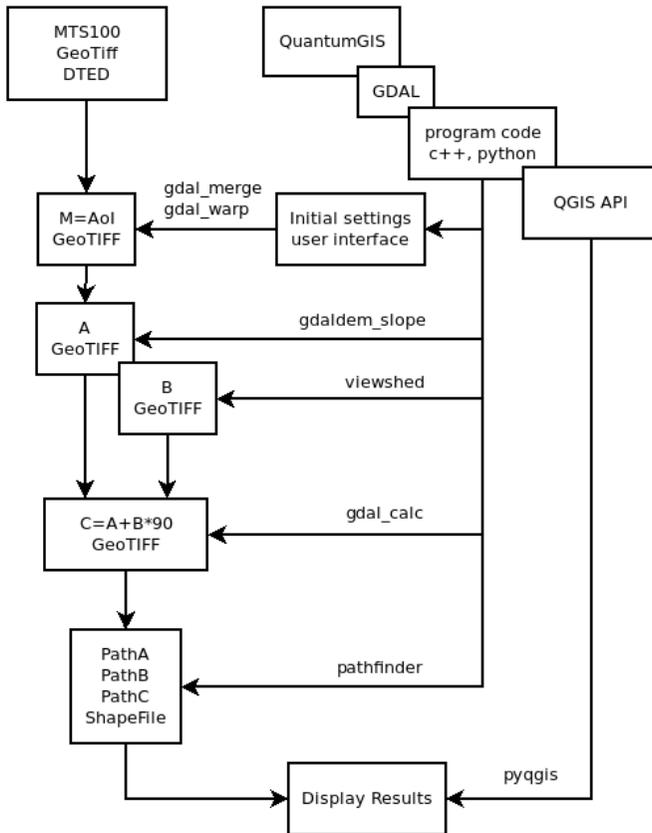
Figure 3: Path planning data flow diagram.
