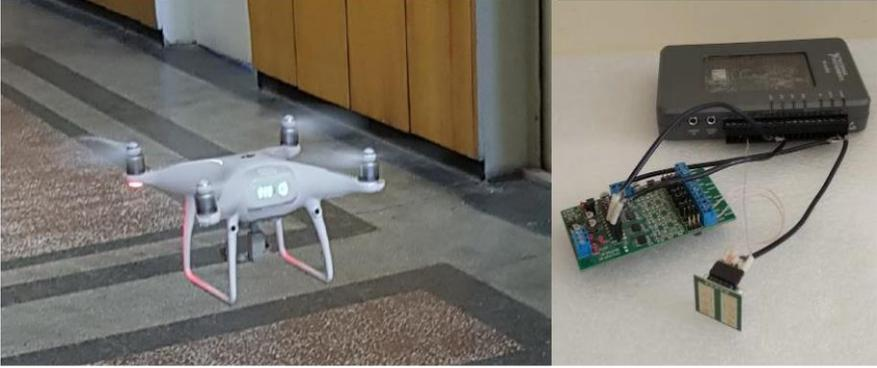
Figure 2: Photos of drone and radar experimental setup.
