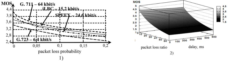
Figure 1: PQoS as a function of (1) packet loss probabilities for different voice codecs<sup>10</sup> and (2) loss rate and delay for SPEEX codec (24,6 kbit/s).<sup>11</sup>
